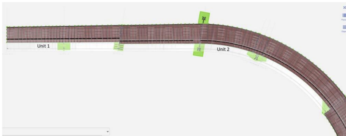
Figure 10. Deconstruction stage of Unit 1 and Unit 2, OpenBrIM Platform FE representation
